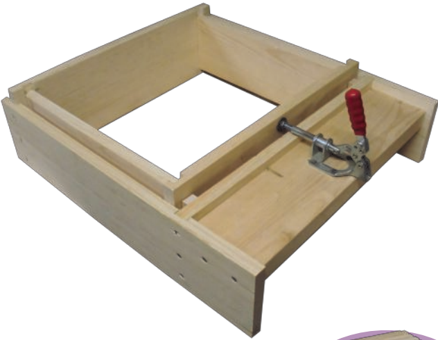
Step 1 Insert End bars and clamp.
