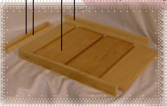
STEP 1: Drive tongue and groove panels together with mallet.
